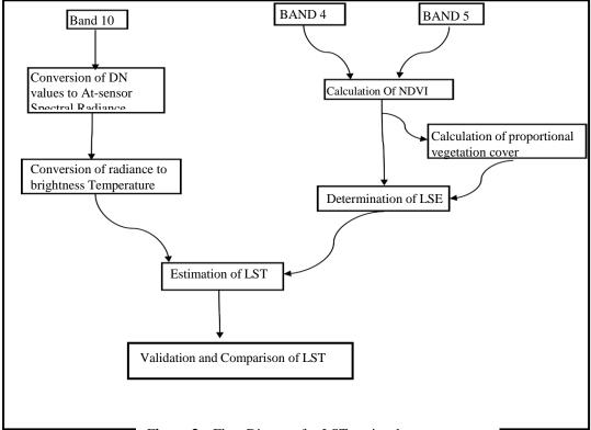
Figure 3 – Flow Diagram for LST retrieval
