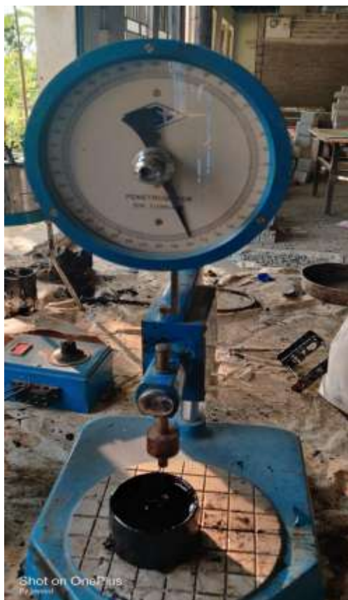
Fig 1: Sample Preparation and Testing of penetration test
