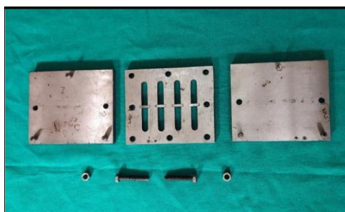
Figure-1 Special Metal Die Used For Tensile Bond Strength Sample Fabrication (Measuring 150 X 100 X 300 MM)
