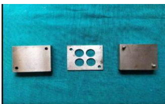
Figure-6 Special Metal Die Used For Anti-Fungal Efficacy Sample Fabrication (Measuring 80 X 60 X 32 MM)
