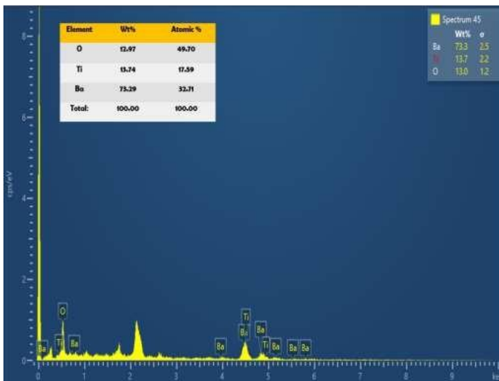
Figure 4. EDX analysis of BTO thin film, inset table shows the percentage composition of Ba, Ti and O
