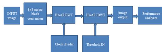
FIGURE 4. Proposed HAAR DWT for image processing application
