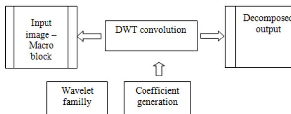
FIGURE 1. General architecture of DWT in image processing
