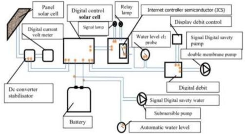
Figure 1: Component of chlorinator
