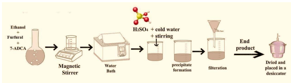
Fig. 2 Schematic diagram showing the (E)-8-((furan-2-ylmethylene)amino)-4-methyl-7-oxo-2-thiabicyclo[4.2.0]oct-4-ene-5-carboxylic acid synthesis process.
