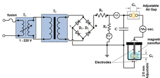
**Figure 1.** A schematic diagram of the electrohydraulic device. The device has a power supply, transformer ( $T_1, T_2$ ), charger resistance ( $R_1, R_2$ ), storage capacitor ( $C$ ), electrodes with adjustable air gap for creating a spark ( $G_1$ ), and submerged electrodes with adjustable air gap for creating a spark ( $G_2$ ).
