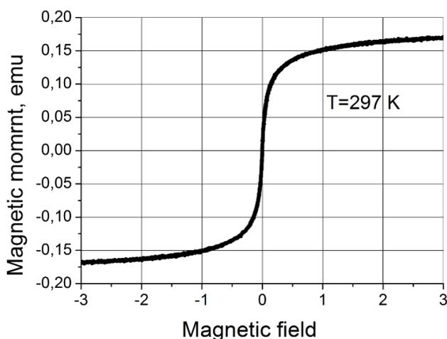
**Figure 3.** The dependence of magnetic moment of electrohydraulically treated bare MNPs on magnetic field
