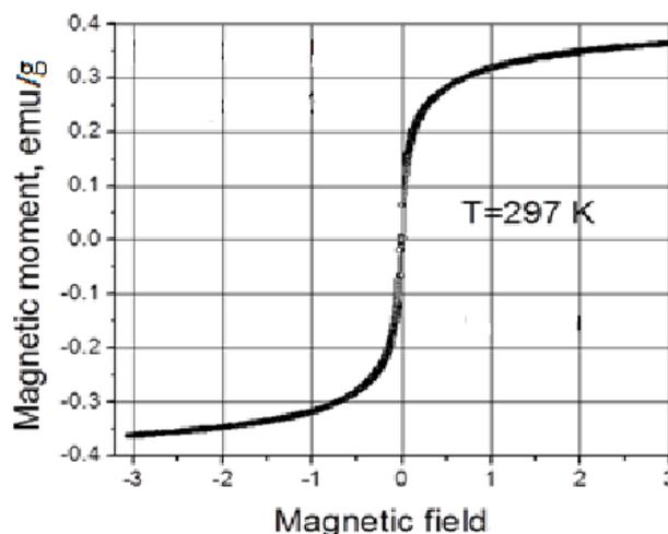
**Figure 5.** The dependence of the magnetic moment of ascorbic acid coated and electrohydraulically treated MNPs on magnetic field.
