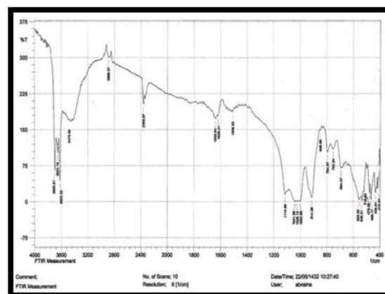
**Figure 1.** FTIR spectrum of al-hussiniyat clay before adsorption.
