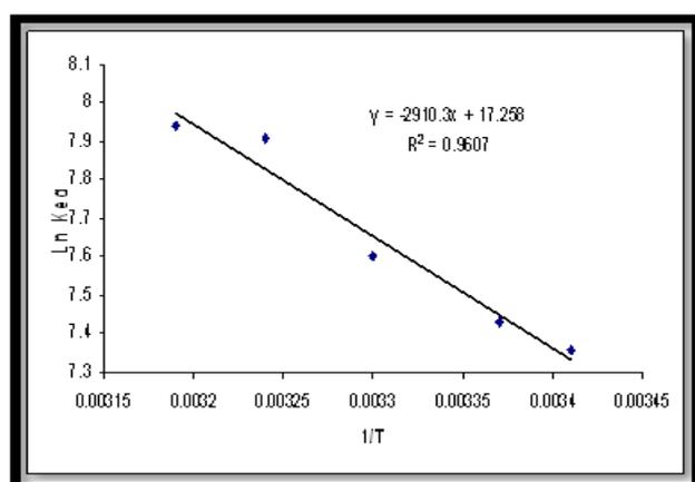
**Figure 6.** Van't Hoff plot of MG adsorption
