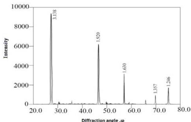
**Figure 4.** X-ray diffraction patterns of standard pure Si.
