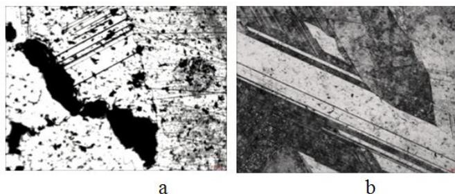
**Figure 1.** Microstructure ( $\times 100$ ) of Si experimental samples of different purity. (a) *n*-MG-Si and (b) pulled with a rate of 0.3 mm  $\text{min}^{-1}$ .
