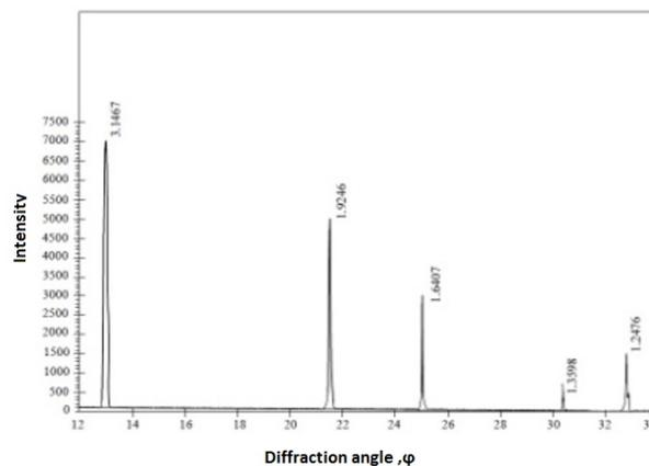
**Figure 3.** The x-ray diffraction pattern of purified pulled Si from MG-Si melt.
