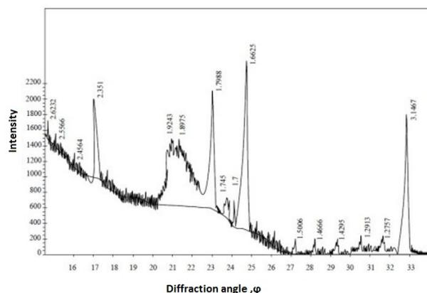
**Figure 2.** The x-ray diffraction pattern of *n*-MG-Si.
