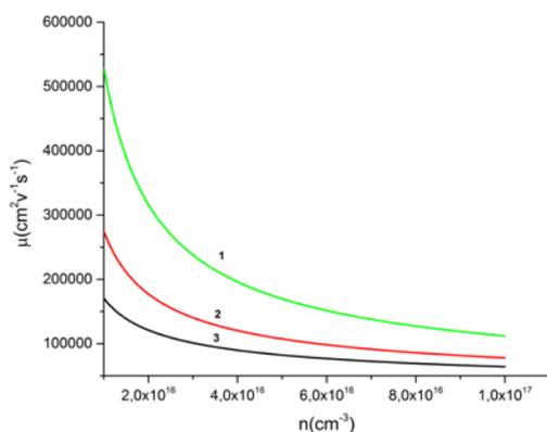
**Figure 1.** Calculated mobility due to scattering of electrons on impurity ions for electron concentration in the range of  $10^{16}$ – $10^{17}$   $\text{cm}^{-3}$  at temperatures: 1 – 300 K, 2 – 150 K and 3 – 77 K.
