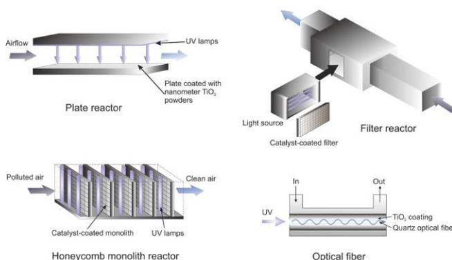
**Figure 5.** Schematic diagrams of various photoreactors for air purification.<sup>74–77</sup>
