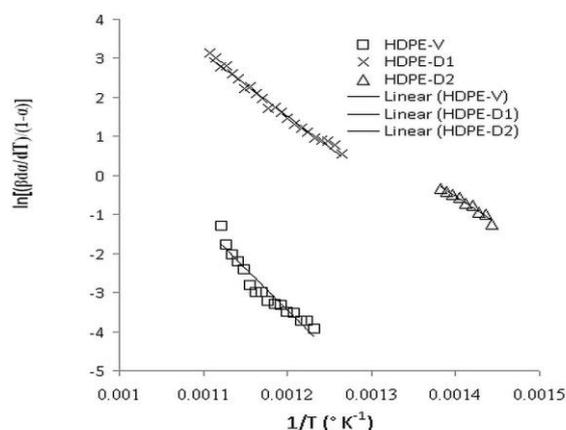
**Figure 5.**  $1/T$  vs.  $\ln[(\beta d\alpha/dT)/(1-\alpha)]$  for virgin and discarded HDPE. Solid lines show the fitting of experimental data to linear models.
